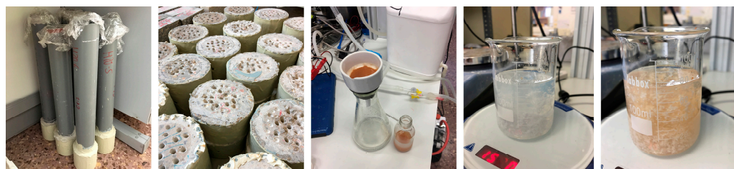
Figure 4. Setup for the chloride diffusion test and the chloride analysis.
