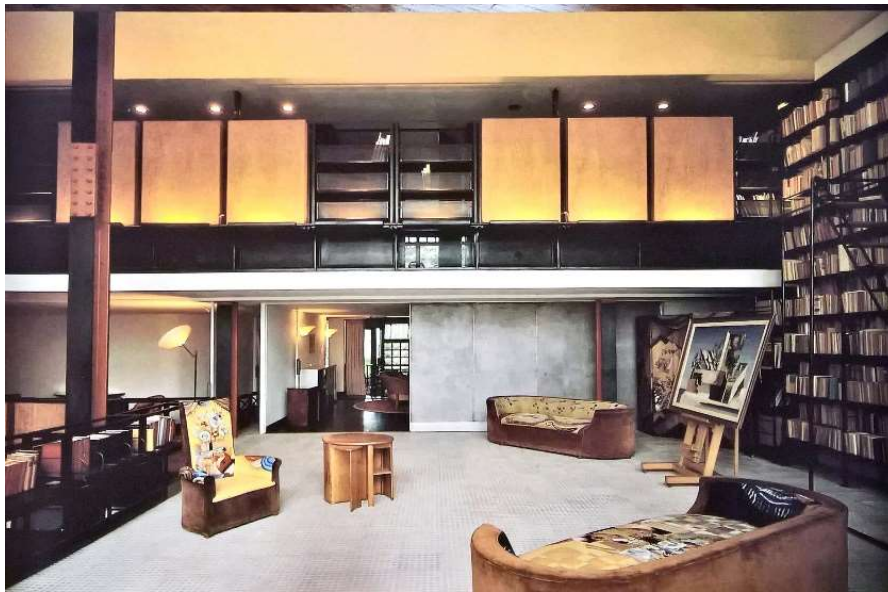
Fig. 5. Maison de Verre, front view of the living room onto the interior garden. On the ground floor the enormous sliding partition can be seen, that allows the room to be configured with continuity from the front to the back facade, or to close off the doctor's working zone, which communicates with the clinic by means of internal stairs. On the upper floor the modular screen is high enough to prevent a direct view of the lower floor, except in the area of the shelf units in the central position, and in a very limited way, as can be appreciated.
