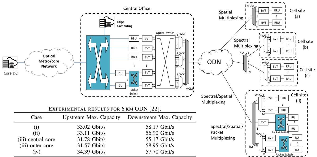
Fig. 3. General scheme for the SDM/WDM DROF fronthaul. Inset table: summary of the experimental results in terms of maximum capacity per flow obtained in [22]. AWG: arrayed waveguide grating; BBU: baseband unit; BVT: bandwidth/bitrate variable transceiver; CU: central unit; DU: distributed unit; MCM: multi-core multiplexer (fan-in/-out); RRU: remote radio unit; RU: remote unit; WSS: wavelength selective switch.
