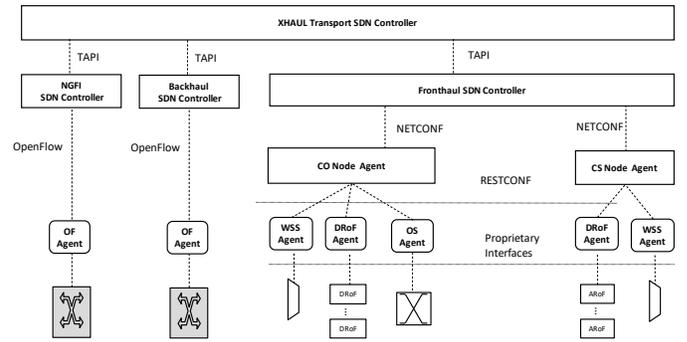
Fig. 4. Transport SDN control architecture.
