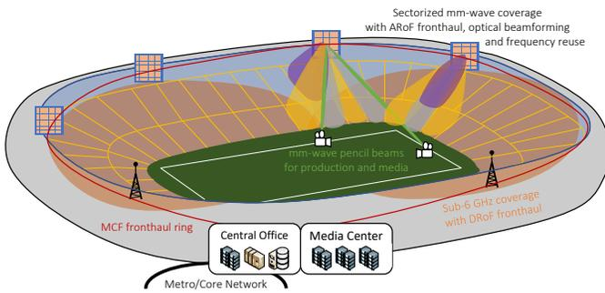
Fig. 2. Multi-service scenario with converged SDM optical fronthaul network, supporting DRoF and ARoF transport as well as optical beamforming.
