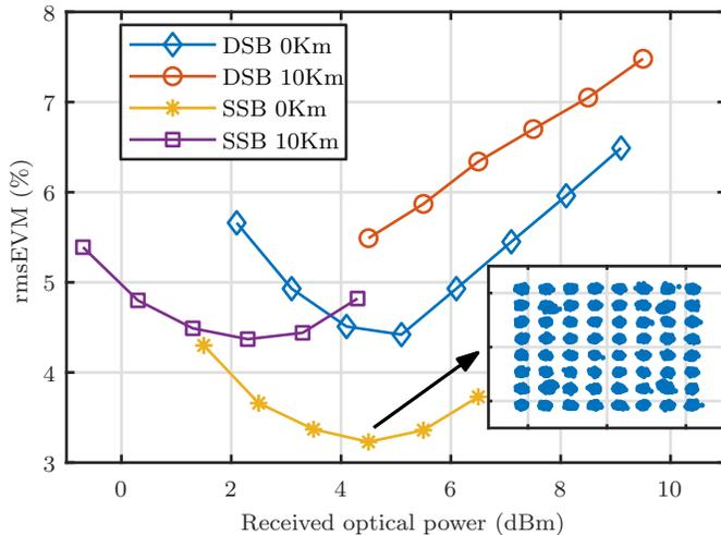
Fig. 7. Experimental results on both setups, EVM as a function of received optical power.
