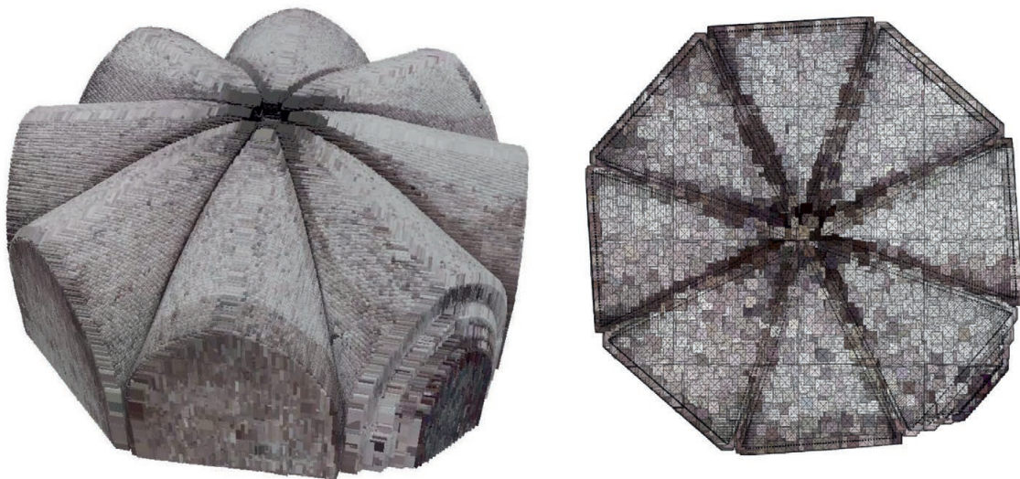
Figure 12 | Model visualization in Esri ArcGIS Pro using the point cloud of the vault and the IFC model.
