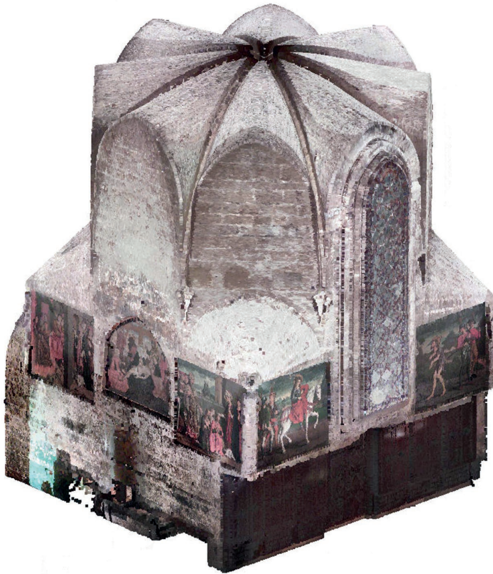
Figure 2 | Point cloud containing 47,073,944 points of the Sacristy Mayor sector of the Metropolitan Cathedral of Valencia.
