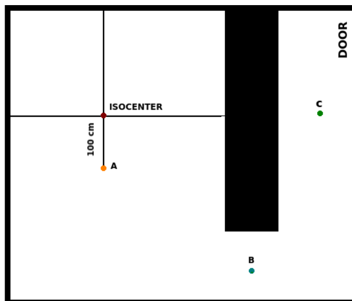
Figure 3. Measurement location points at the radiotherapy facility of a Varian Clinac at the “Hospital Universitari I Politècnic La Fe de València”.
