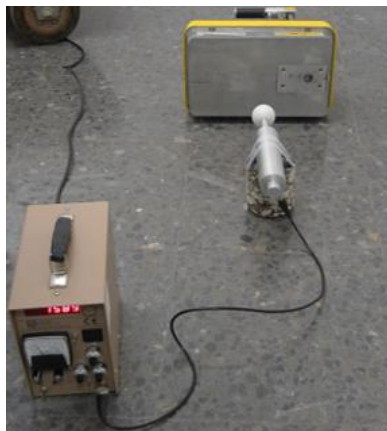
Figure 6. ^{241}\text{Am-Be} neutron source measuring experimental set up with the BSS system
