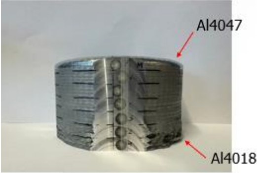
Figure 16. LIBS sample with Al alloy and Si gradient over the height.
