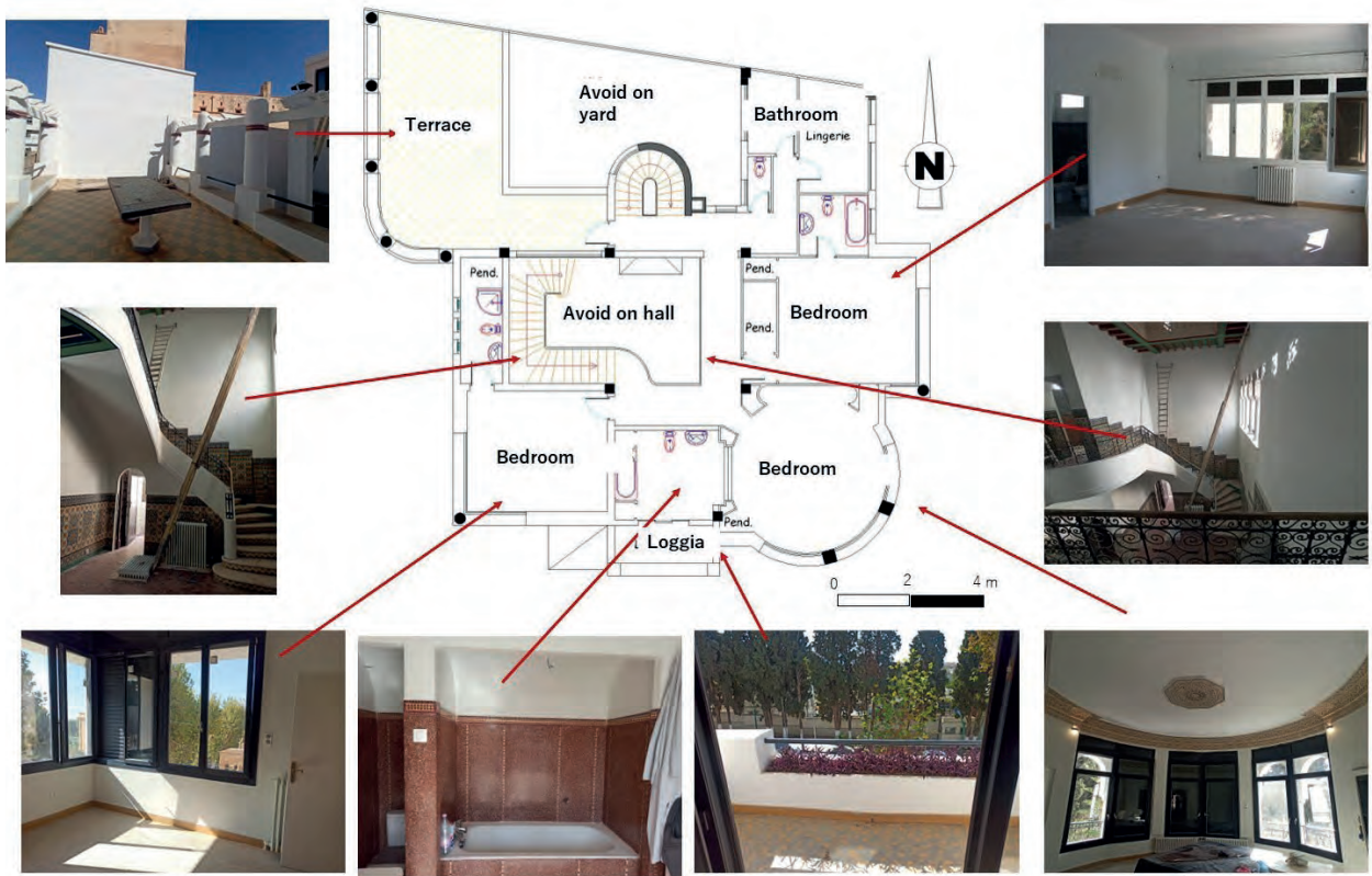
Fig. 18. First floor plan of the villa The Moghrébine. (source: archive of APC of Tlemcen developed by the authors).
