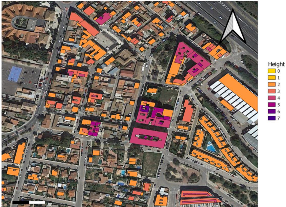
Fig. 3. Graphic illustration of the effects of filtering out spatial polygons of less than one height and less than 20 m 2 in one municipality of the 2 nd ring (San Antonio de Benagéber). Note the significant number of buildings discarded. Source: Own elaboration with QGIS.
