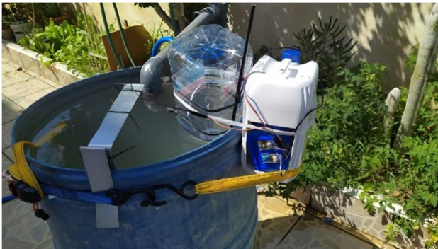
Fig. 5 Sensor node in a plastic drum with river water sample
