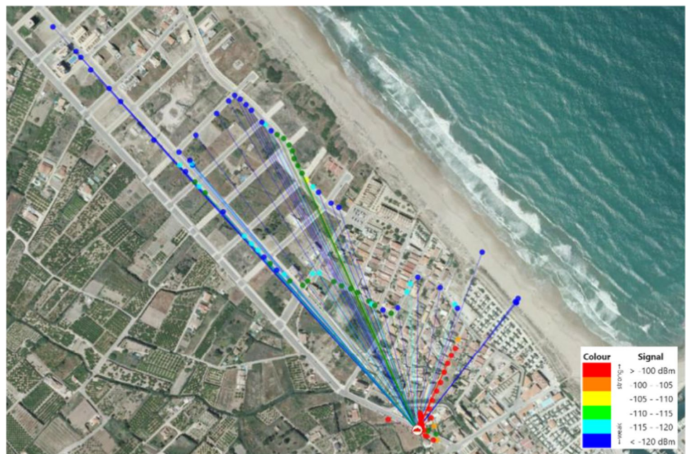
Fig. 7 Values of RSSI measured for The Things UNO module
