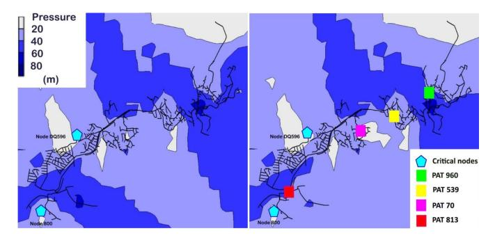
**Figure 12.** Pressure contour map for network 8–12 statistics maximum from EPANET. Initial network (left contour) and network with PATs (right contour).
