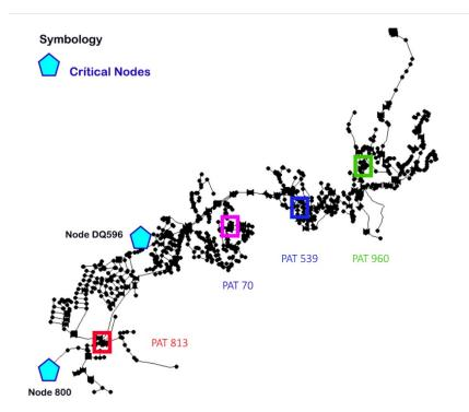
Figure 8. PAT location and critical nodes obtained by the methodology described.
