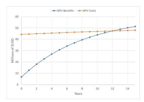
**Figure 11.** Payback period is represented by the intersection point where NPV benefits overpass NPV costs.
