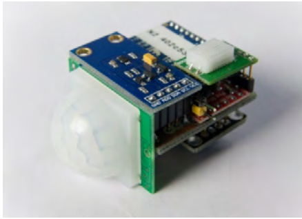
Figure 1 Sensor nodes: a, gateway node, b, passive sensor node
