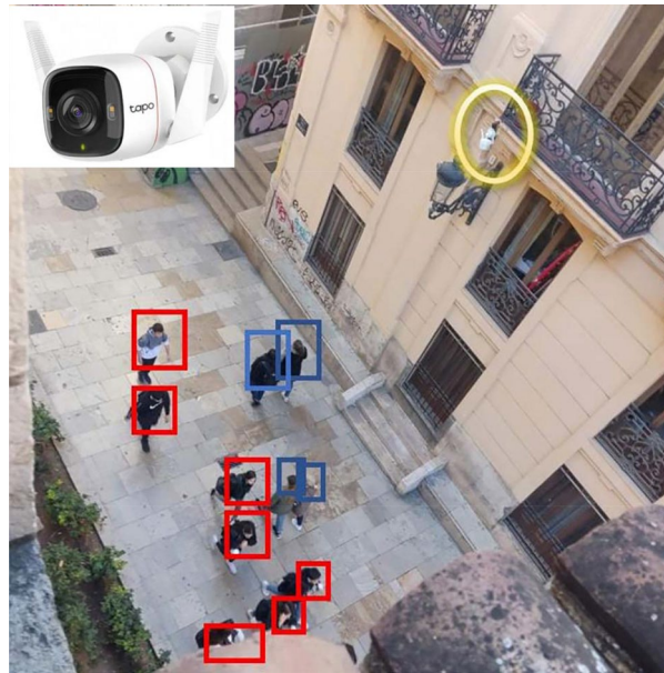
Figure 3. Detection of the flow of people with the CPF-SENSOR video camera in Miguelete street.
