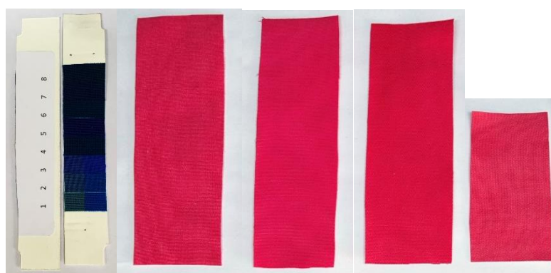
Figura 35. Rasq. rPVB/PAC 150 g/l -10 g/l pig; Impreg. rPVB/PAC 150g/l- 10 g/l pig
