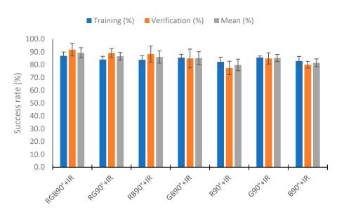
Figure 21. Success rate in the neural network with the data at 90° of the RGB light and IR light.
