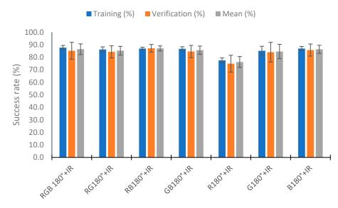
**Figure 23.** Success rate in the neural network with the data of the different RGB light at 180° and IR light.
