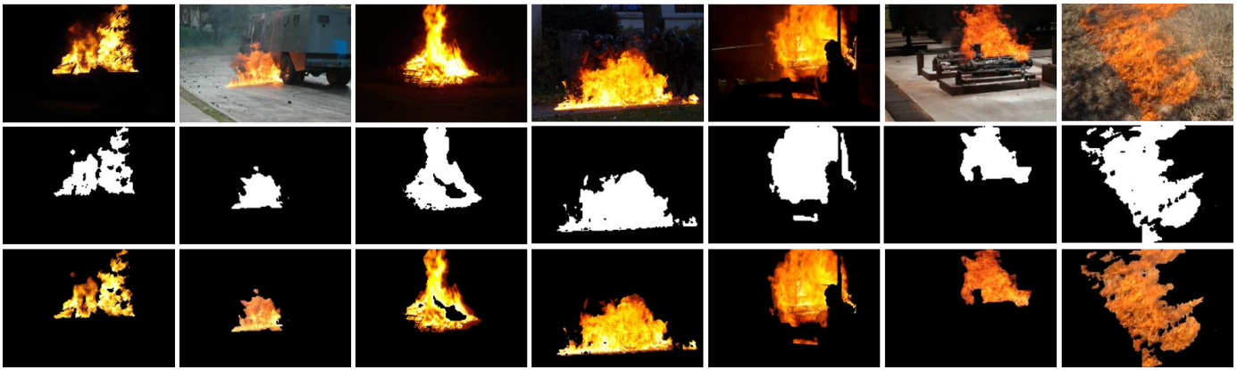
Fig. 3. Visual results obtained by our method for fire-specific region extraction, where the first row represents input images and the second and third rows contain segmentation and fire-specific region extraction results, respectively.
