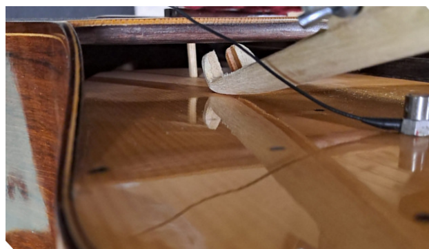
Figure 1: Soundpost mounted between the two top plates with its setter tool.
