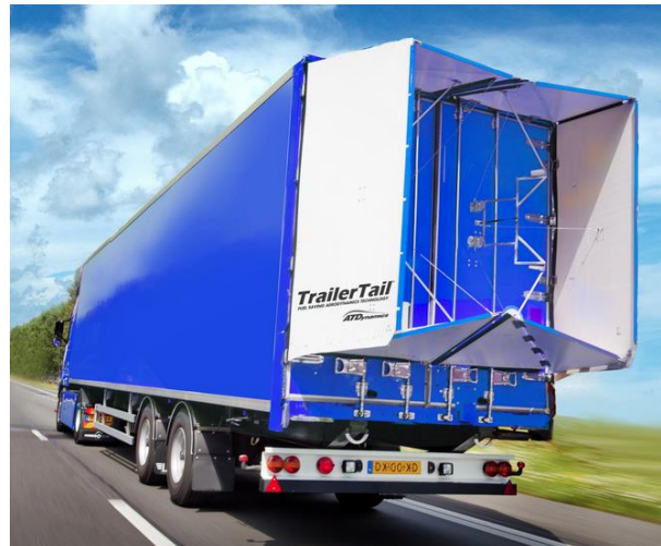
Figure 2: Drag Reduction System: Lorry on road with DRS implemented [ICIL].
