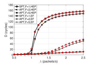
Figure 9: Delay for different packet arrival rates.
