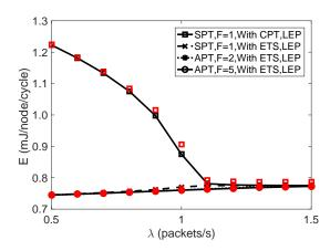
Figure 14: Energy consumed by the RN per cycle with and without ETS.
