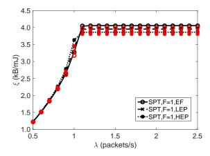
Figure 8: Energy efficiency of SPT (F=1) for different packet arrival rates.
