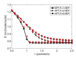
Figure 12: Energy consumption for different packet arrival rates.
