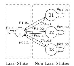
Figure 3: A frame-level error model for error-prone channels with one state in the loss macrostate and three states in the non-loss macro-state.
