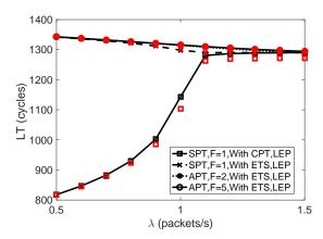
Figure 16: Lifetime of the RN with and without ETS.
