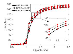
Figure 5: Delay of SPT (F = 1) for different packet arrival rates.
