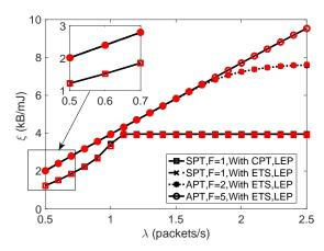
Figure 15: Energy efficiency of the RN with and without ETS.
