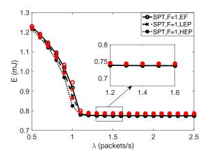
Figure 7: Energy consumption of SPT (F = 1) for different packet arrival rates.
