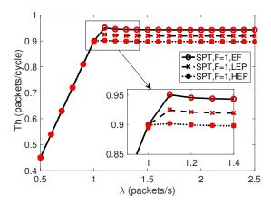
Figure 4: Throughput of SPT (F=1) for different packet arrival rates under different channel conditions.
