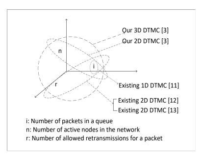
Figure 2: Illustration of the DTMC models for DC MAC protocols: existing versus ours.
