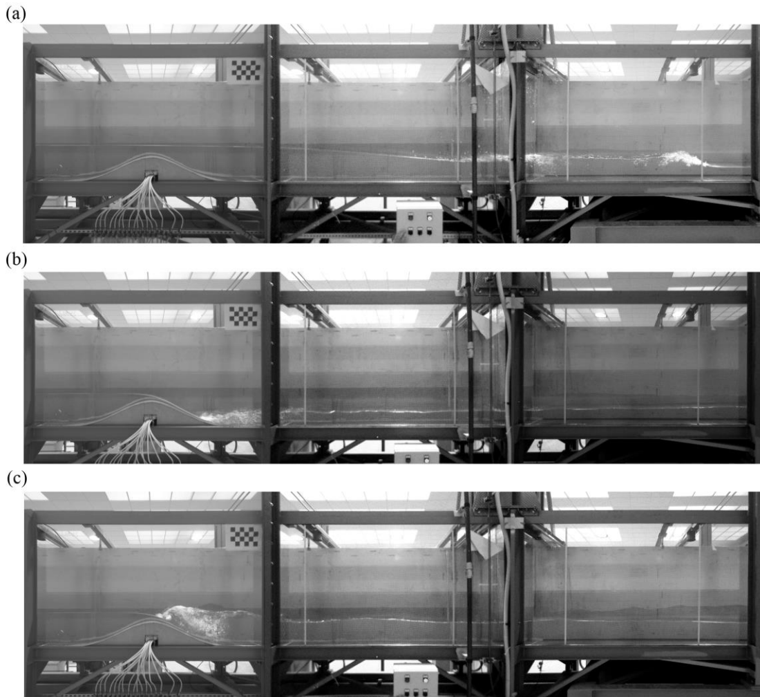
226 227 Fig. 3. Panoramic views of cameras 4, 5 and 6 (from left to right) for test 1 at: (a) t = 228 1 s, (b) t = 6 s, and (c) t = 10 s. The piezometric tubes are shown in the left images.
