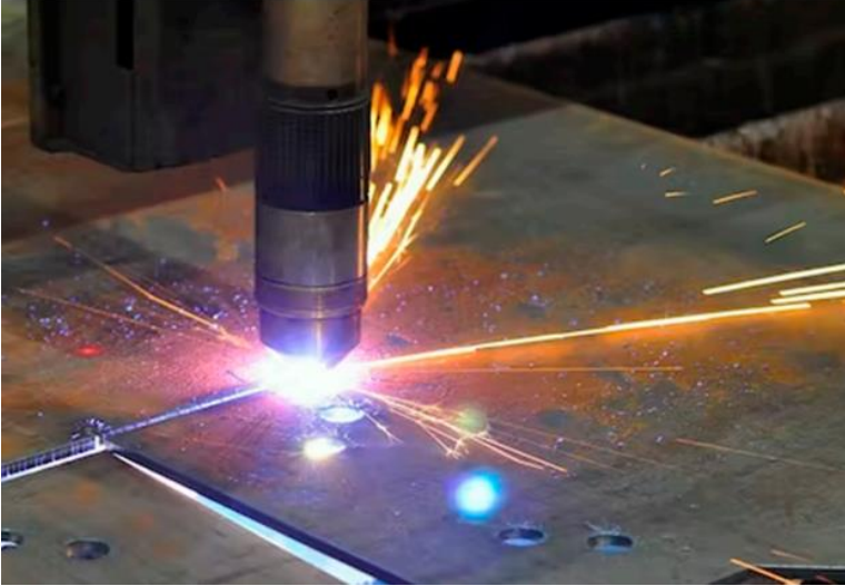
Figure 26. Material preparation using computer numerical control (CNC) plasma sample (case study 1).
