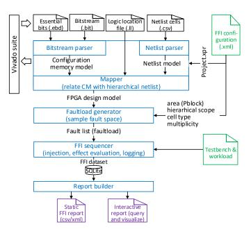
Fig. 1. Workflow and main components of the BAFFI tool
