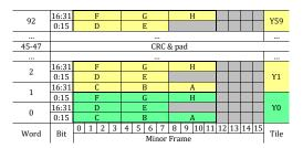
Fig. 4. Location of LUT content in the CM of Ultrascale+ FPGA (8 LUTs per CLB slice labeled A–H)
