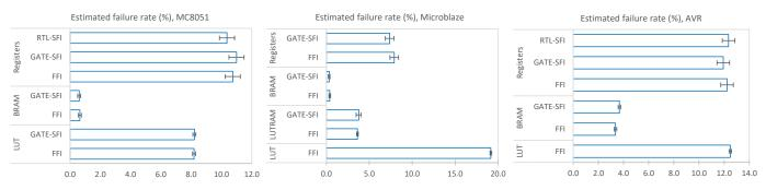
Fig. 9. Dependability estimates of three considered DUTs, obtained by RT-level SFI, gate-level SFI, and FFI experiments
