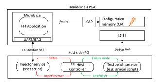
Fig. 6. FFI setup controlled by host-side FFI application
