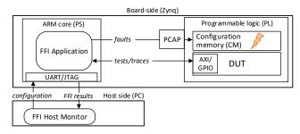
Fig. 5. FFI setup controlled by board-side FFI application
