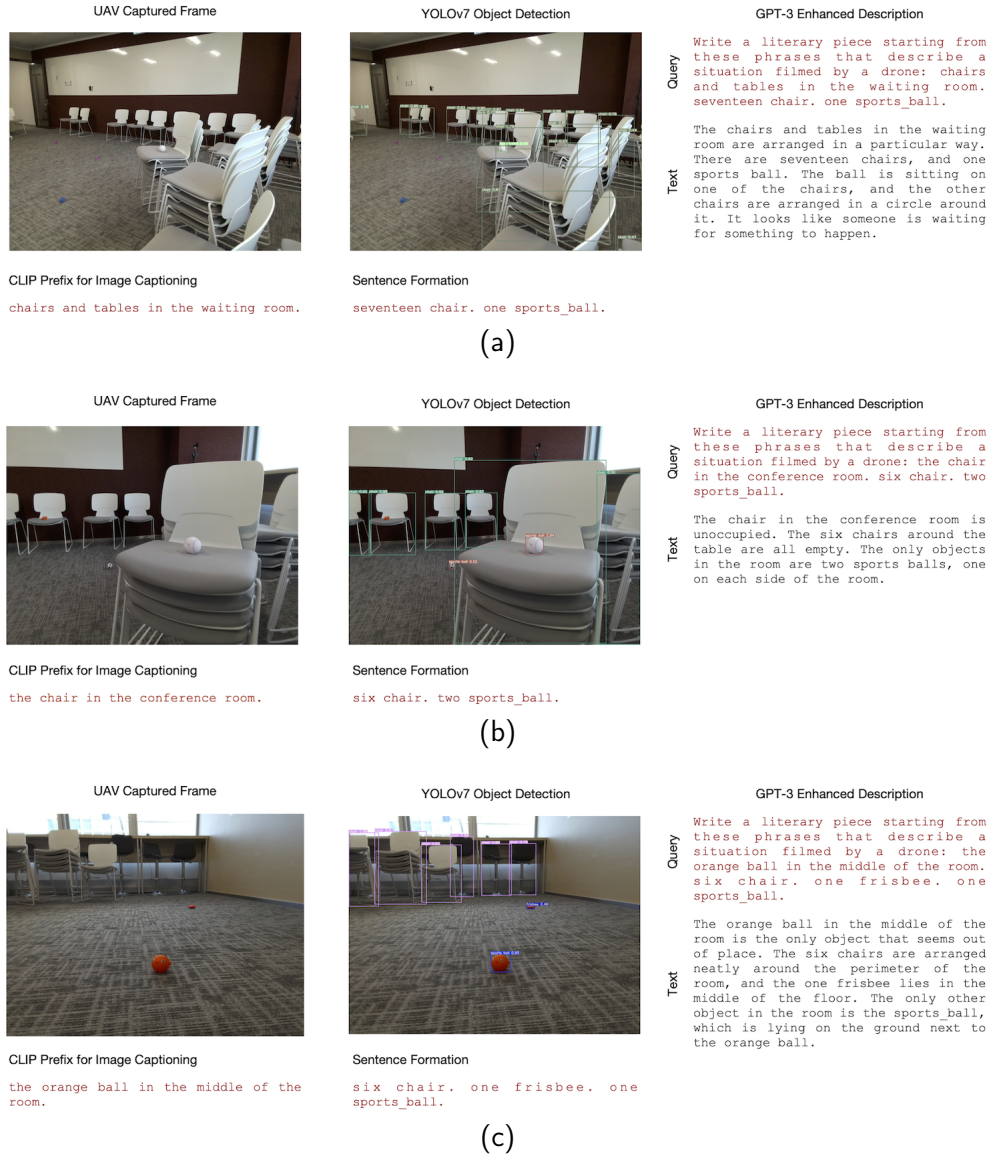
Figure 3.3: UAV captured frame processing and GPT-3. Very good GPT-3 descriptions of the scene.
