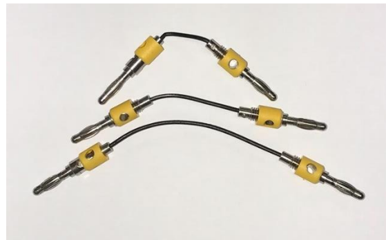
Figure 5. The 20, 40, and 80 mm test specimens connected to the banana probes.
