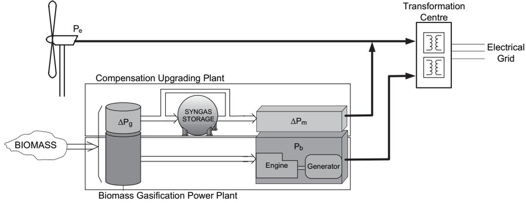
Fig. 2. Proposed hybrid wind-biomass system.
