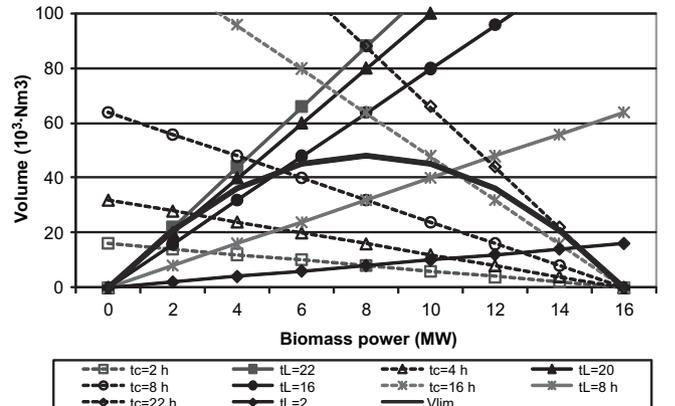
Fig. 4. Storage volume ( $f = 0.1$ ,  $P_e = 40 \text{ MW}$ ,  $r_g = 0.25$ ).
