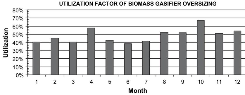
Fig. 10. Evolution of the utilization factor of the oversized gasifier along the year.
