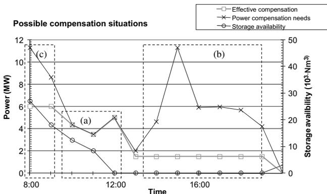
Fig. 11. Different compensation situations in a critical day: (a) Total compensation, (b) Storage tank is empty, and (c) Maximum compensation capacity of 6 MW.
