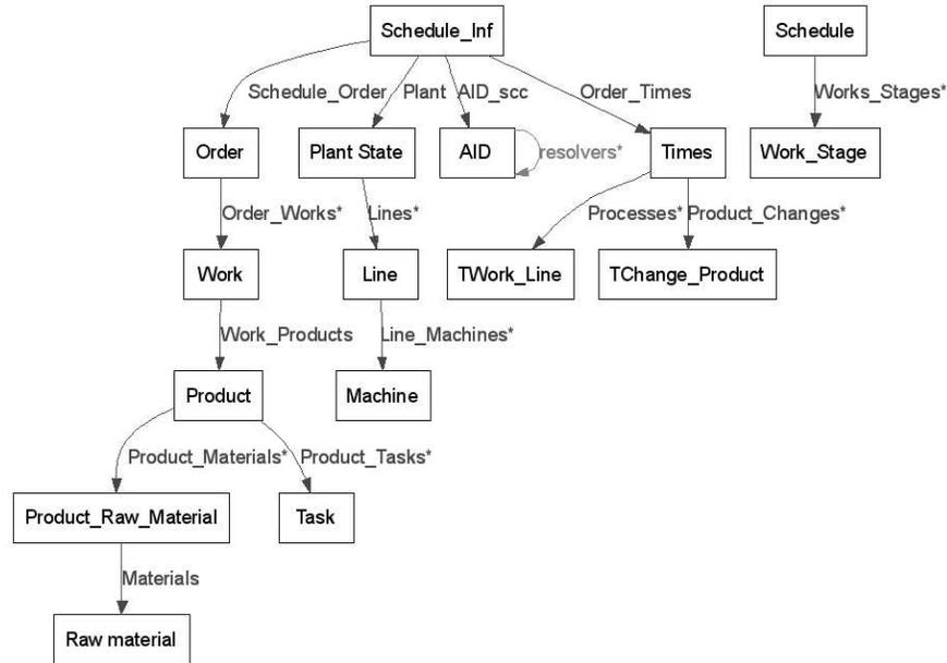
**Fig. 5.** Ontology concept example for the production scheduling of a ceramic tile factory
