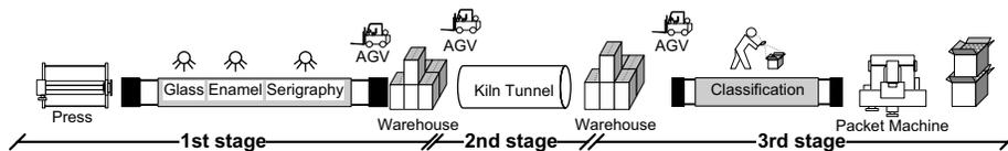
**Fig. 4.** Ceramic Tile Production Process: three stage hybrid flow shop
