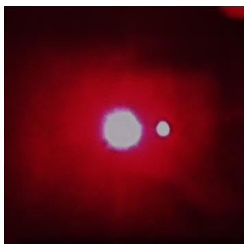
Figure S5. Diffraction pattern projected on a white screen of biofunctionalized VTG hydrogel functionalized with the thiolated probe after its hybridization with 2 \mu\text{M} of the complementary target and washing with SSC1x. VTG was surrounded by SSC1x and illuminated with the probe laser beam at 633 nm.
