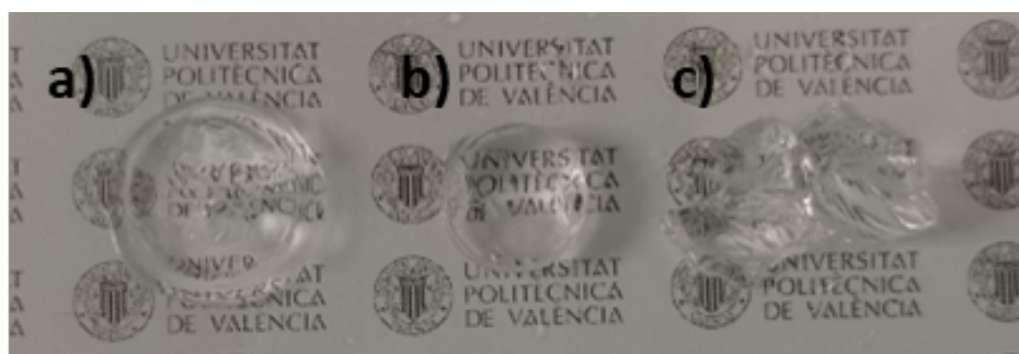
Figure S2. Digital images of hydrogels pieces with different compositions and consistency AM(8)/PA_0.050, soft; b) AM(8)/PA_0.250, adaptable and c) AM(32)/PA_0.250, brittle.
