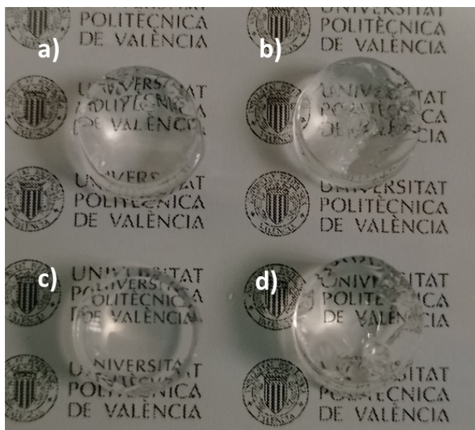
Figure S3. Digital images of selected hydrogels pieces with different compositions a) AM(8)_0.250, b) AM(25)/PA_0.050 c) AM(8)/PA_0.250, and d) AM(25)_0.250.
