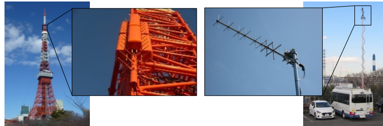
Figure 2.14 Transmit antenna (left) and receive antenna (right) used for field experiments in Section 5.1.
