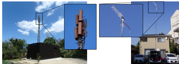
Figure 2.15 Transmit antenna (left) and receive antenna (right) used for field experiments in Section 5.2.
