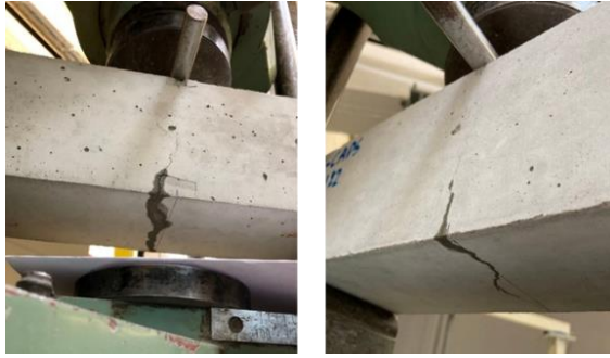
Figure 8-5. Successful rupture of embedded capsules by releasing the sealing agent through the crack
