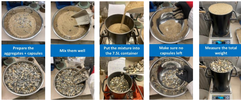
Figure 8-16. Schematic procedure of LBD test on a single type/fraction of aggregate
