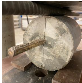
Figure 5-2. Splitting the pull-out specimen by means of a Brazilian splitting test
