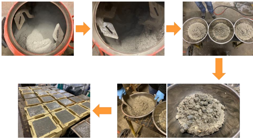
Figure 8-38. Procedure of casting capsule-based concrete
