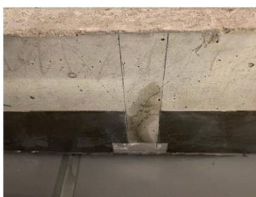
Figure 7-11. Comparison of water ingress in the cracked reference and MIC concretes (both pictures were taken 15 min after the capillary water absorption test was performed)
