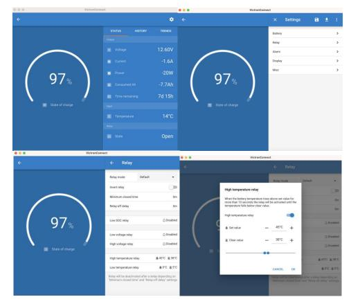
Figure 21. Configuration of conditions based on temperature sensor and relay of the BMS-712.
