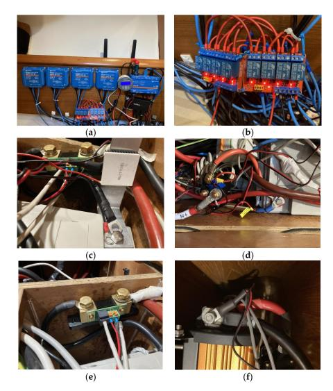
**Figure 23.** Experimental set-up. (**a**) The 4 solar chargers, the Cerbo GX, the BMV-712 monitor, and the two 4-relay modules. (**b**) The two 4-relay modules. (**c**) The Peltier cell for the induction of threshold temperature values. (**d**) The power relay controlled by the BMV-712 temperature-monitoring sensor. (**e**) The shunt of the BMV-712 device. (**f**) Temperature Sensor 25 connected to the inverter.
