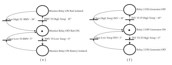
**Figure 15.** (a) Start/stop generator by Temperature Sensor 24 PN Model. (b) Start/stop generator by Voltage PN Model. (c) Start/stop generator by Current PN Model. (d) Start/stop generator by SOC PN Model. (e) Connection/disconnection of battery by BMV Temperature Sensor PN Model. (f) Start/stop generator by Temperature Sensor 25 PN Model.
