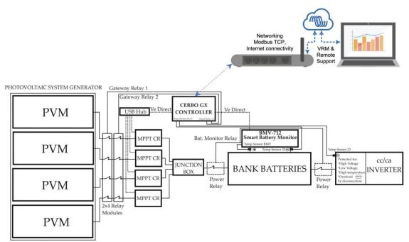
Figure 1. Photovoltaic generation system with integrated and distributed smart BMS system.
