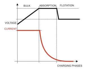
Figure 7. Batteries' three-phase charge process.
