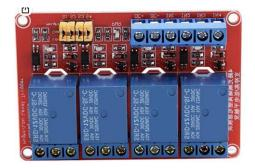
Figure 6. Photovoltaic generation system: 4-relay modules of on/off actuator.
