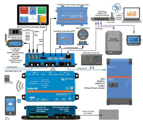
Figure 12. Cerbo GX cloud networking devices configuration.
