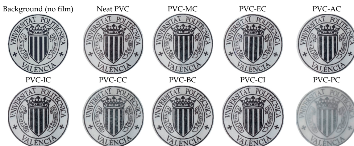
Figure 5. Optical images showing the transparency of films of the neat PVC and plasticized PVC films with the different cinnamic acid-based esters.
