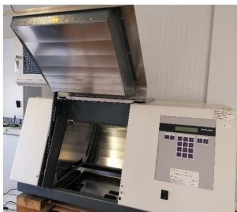
Figura 6. Simulador solar SUNTEST XLS+ (Atlas Material Testing Solutions).
