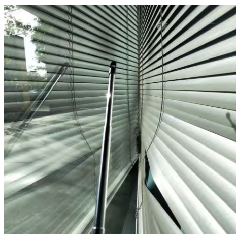
Figure 7. On-site measurements of the indoor dry-bulb temperatures between the glass and the curtain, at 13:00 h in the summer's hottest week (18–22 July).
