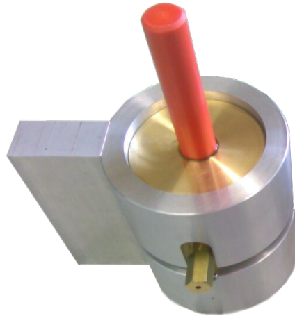
Figure 5.10: Manufactured prototype of the 11 GHz split-cylinder-cavity resonator.
