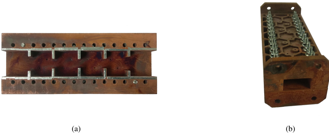
Figure 3.14: Manufactured prototype of the WR75 filter: (a) Top view of the body part showing the filter cavities and coupling irises. (b) Assembled filter showing the waveguide flange.
