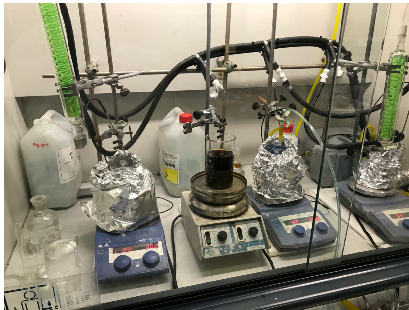
Figure 3.2: (a) Schematic of the electroless plating process. (b) Experimental setup for the electroless plating.
