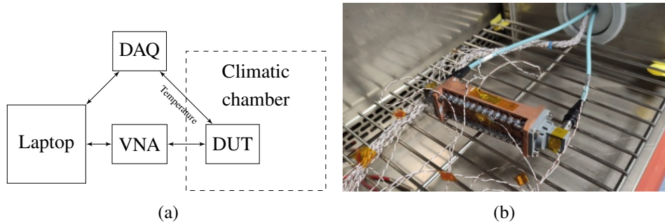
Figure 3.42: (a) Measurement setup diagram for vacuum temperature tests. (b) WR75 filter inside the climatic chamber.
