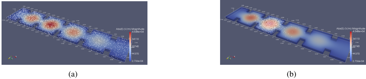
Figure 3.57: Distribution of electrons population in the low-profile filter for an 10.775 GHz input signal with a power of 400 W. (a) Initial distribution of 3000 electrons. (b) Electron distribution after 80 nsec. Electrons are depicted in white over the electric field distribution of the filter.
