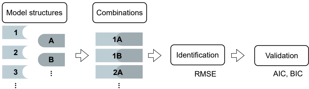
Figure 8.2: Pramlintide models selection procedure summary. Different model structure candidates are assembled to form model combinations that are identified based on the RMSE, and the most adequate model is selected based on the validation AIC and BIC results.
