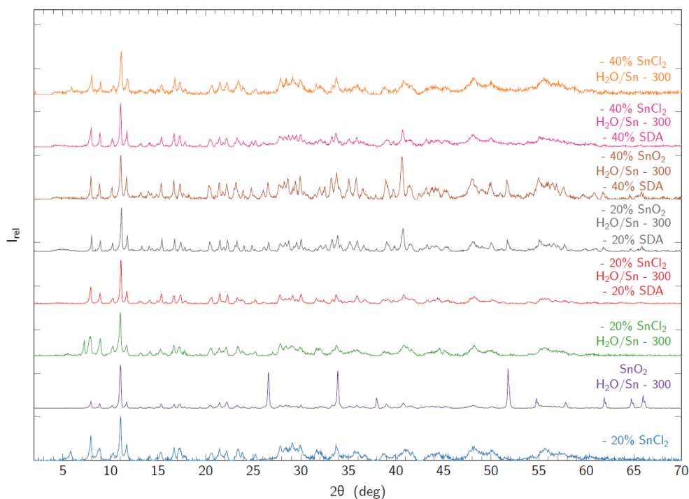
Figure B.5: PXR D patterns of IZM-5 with a reduced SnCl 2 molar content by 20% (in blue), with SnO 2 and Sn source and increased H 2 O/Sn molar ratio to 300 (in purple), with a reduced SnCl 2 molar content by 20% and increased H 2 O/Sn molar ratio to 300 (in green), with a reduced SnCl 2 molar content by 20%, increased H 2 O/Sn molar ratio to 300 and reduced SDA molar content by 20% (in red), with a reduced SnO 2 molar content by 20%, increased H 2 O/Sn molar ratio to 300 and reduced SDA molar content by 20% (in grey), with a reduced SnO 2 molar content by 40%, increased H 2 O/Sn molar ratio to 300 and reduced SDA molar content by 40% (in brown), with a reduced SnCl 2 molar content by 40%, increased H 2 O/Sn molar ratio to 300 and reduced SDA molar content by 40% (in pink) and with a reduced SnCl 2 molar content by 40% and increased H 2 O/Sn molar ratio to 300 (in orange)
