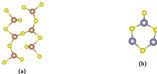
Figure 2.26: Representation of (2.26a) \text{Sb}_3\text{S}_6 and (2.26b) \text{Sn}_3\text{S}_4 building units [146] [147]
