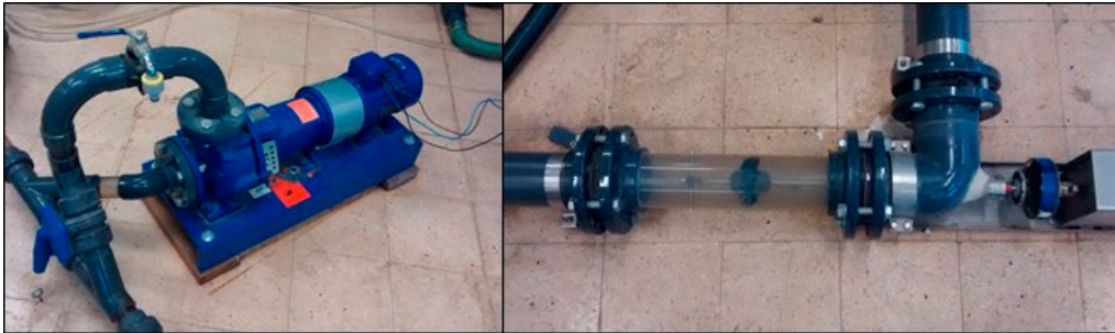
Figure 6. Hydraulic machines at IST-Universidade de Lisboa: PAT (left); and tubular propeller (right).
