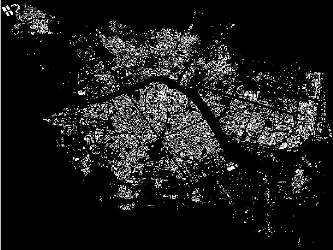
Figure 12: Final mask or GEO_MASK_WS delivered by the ROOFTYPEDETECTION.m MATLAB code. This mask does not consider the slope of the buildings.
