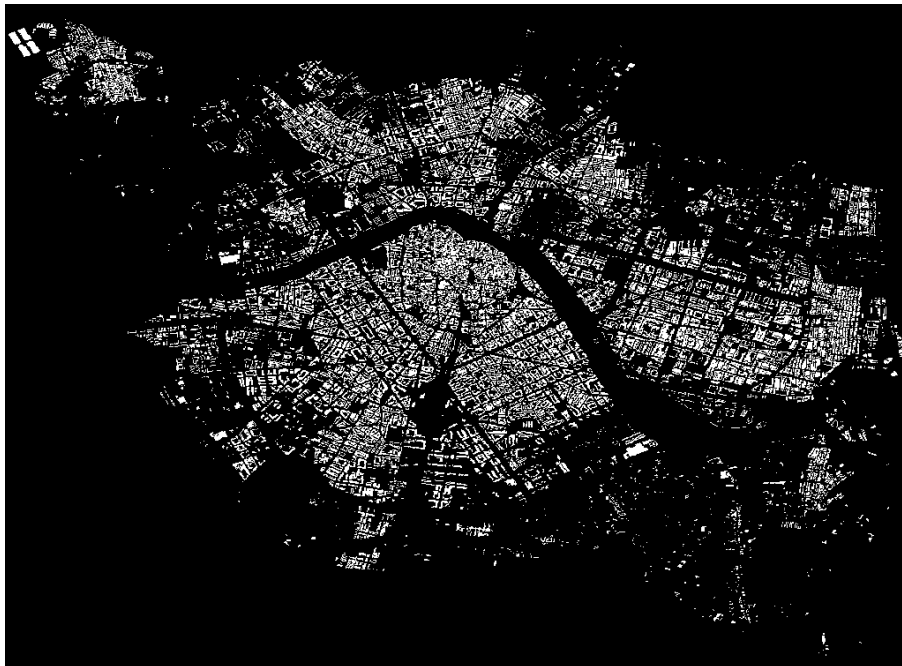
Figure 24: "GEO_MASK". Binary mask representing the buildings considered with potential for GR assembly by the AV developed within the MATLAB code.
