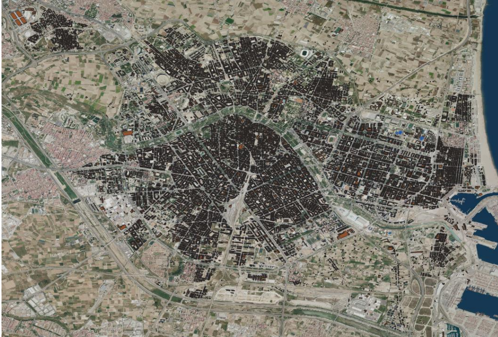
Figure 26: "GEO_MASK_CADASTRAL_VALENCIA". Vector layer corresponding to the superposition of the layer "GEO_MASK_VECTORIAL" on the layer "ValenciaUrbano_PartInfo" obtained in section 3.3.2.
