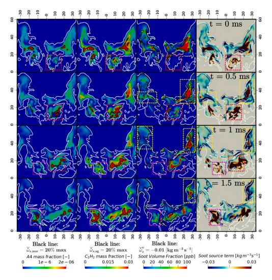
Fig. 12. Temporal sequence of A4 mass fraction,  $C_2H_2$  mass fraction, SVF and soot source term contours. White line: stoichiometric mixture fraction isoline. Black lines: isolines of soot source terms. Spatial units in mm. (For interpretation of the references to color in this figure legend, the reader is referred to the web version of this article.)
