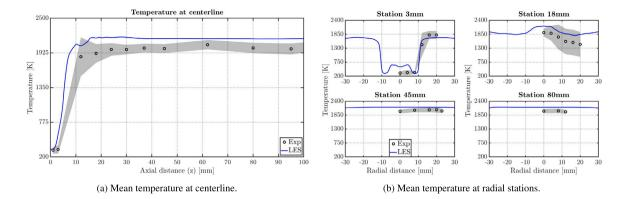
Fig. 16. Comparison between LES results and experiments (Op 2) of temperature. Shaded area: standard deviation of measured temperature.
