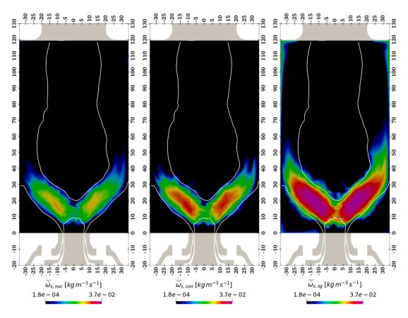
Fig. 13. Time-averaged contours of soot production source terms by subprocess. Left: nucleation. Center: condensation. Right: surface growth. White line: stoichiometric mixture fraction isoline. Legend in log scale. Spatial units in mm. (For interpretation of the references to color in this figure legend, the reader is referred to the web version of this article.)
