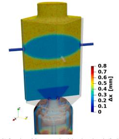
(b) Overview of the computational domain and mesh (Op 1). etup [21]. Colors: cell size in mm.
