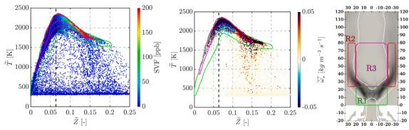
(a) Scattered plot of mixture fraction  $(\widetilde{Z})$  and temperature (b) Scattered plot of mixture fraction  $(\widetilde{Z})$  and temperature  $(\widetilde{T})$  with solid lines representing different regions of the burner. Colors: Soot Volume Fraction. burner. Colors: total soot source term  $(\widetilde{\omega}_s^c)$ .
