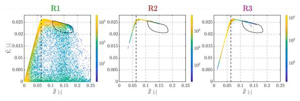
Fig. 10. Scattered plots of mixture fraction and progress variable from instantaneous LES results. Colors: joint-PDF of  $\widetilde{Z} \cdot \widetilde{Y_c}$ . Black line: isoline of  $\widetilde{\phi}_s^c = 0.05 \text{ kg/m}^3 \text{s}$ .
