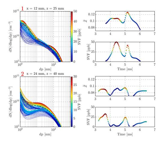
Fig. 14. Instantaneous and time-averaged PSD results (Op1) at two different locations inside the combustion chamber (see markers in Fig. 7). Left: instantaneous (solid lines) and time-averaged (black dashed line) PSDF. Right: time-evolution of mixture fraction ( $\widetilde{Z}$ ) and SVF. Colors: instantaneous SVF magnitude.
