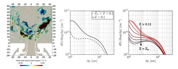
Fig. 15. Spatial-averaged PSD results (Op1). Left: contour of total soot source term in a vertical cut plane. Green line: Z = 0.1 isoline, white line:  $Z = Z_{st}$  isoline. Center: PSDF in two regions depending on Z. Right: evolution of the PSDF from very rich conditions to  $Z_{st}$ . (For interpretation of the references to color in this figure legend, the reader is referred to the web version of this article.)
