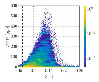
Fig. 11. Scattered plot of mixture fraction and SVF from instantaneous LES results. Color: joint-PDF of  $\widetilde{Z}$ -SVF.
