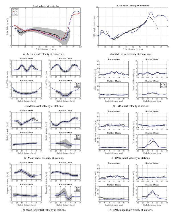
Fig. 4. Comparison between LES results (non-adiabatic case) and experiments of velocity field. Shaded area: RMS velocity fluctuation from FoV experiments.
