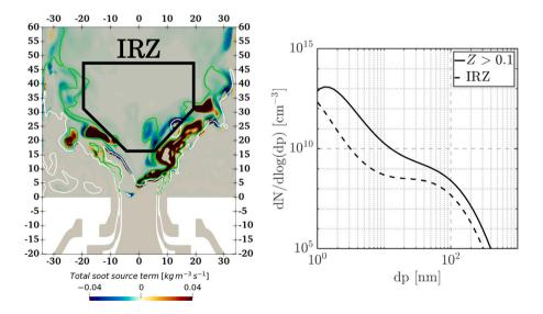
Fig. 20. PSD results for Op2. Left: contour of total soot source term in a vertical cut plane. Green line: Z = 0.1 isoline, white line:  $Z = Z_{st}$  isoline. Right: spatial averaging of PSDF in two regions: rich region (Z > 0.1) and IRZ. (For interpretation of the references to color in this figure legend, the reader is referred to the web version of this article.)
