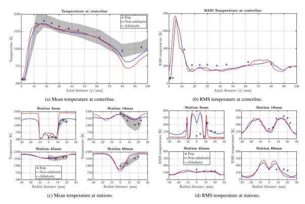
Fig. 6. Comparison between LES results (adiabatic and non-adiabatic) and experiments of temperature field. Shaded area: RMS of the measured temperature.
