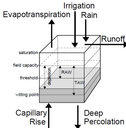
Fig. B2.1. Water balance at the root zone (From Allen et al., 1998).
