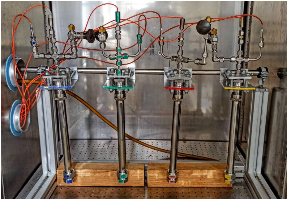
Figure 6.1: Miscibility test bench
