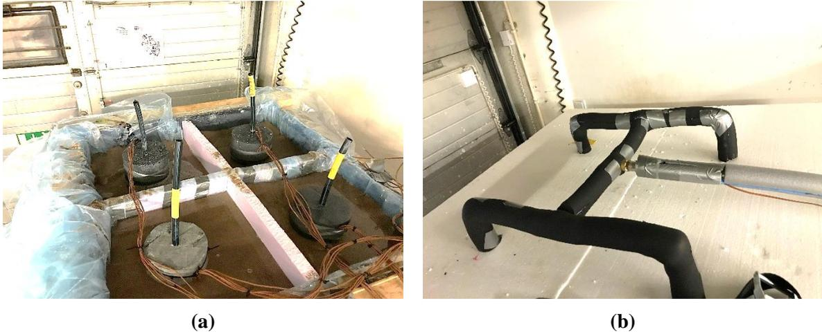
**Figure 5-7: The four-column test setup: (a) Four separated columns filled with sand and saturated with water, and (b) Connection of the grout columns to the circulation pump.**
