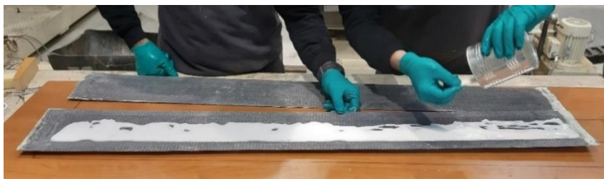
Figure 5. Fill and glue two blade halves
