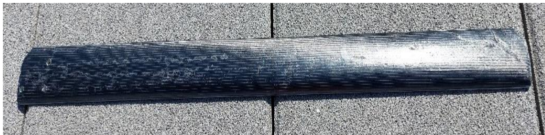
Figure 6. Small recyclable wind blade WB-AKE-1
