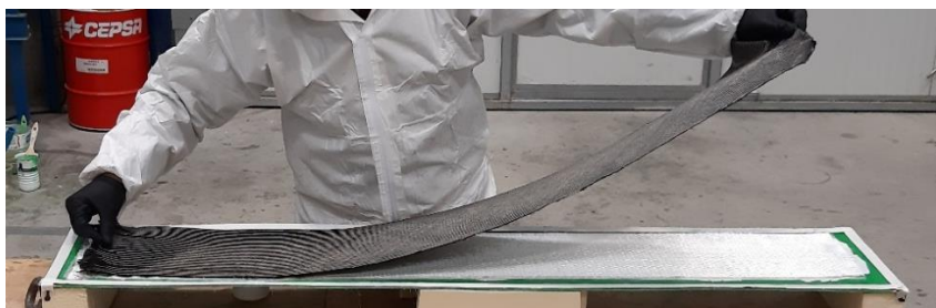
Figure 3. Lay-up fibres in the molds
