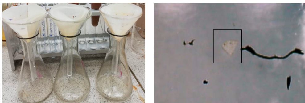
Figure 8. Density separation of plastic particles from soil leachate.
