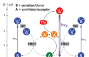
Scheme 4 Photon upconversion technology based on TTA. After the absorption of low-energy photons ( h\nu_1 ), a sensitizer triplet is produced by intersystem crossing (ISC) from its singlet. Subsequently, TTEnT from sensitizer triplets to the acceptor (Dexter mechanism) occurs. When two acceptor molecules in their triplet states are capable of colliding during their lifetimes, a higher singlet energy level is formed by TTA and, consequently, generates delayed upconverted fluorescence ( h\nu_2 ).
