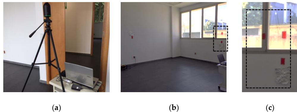
Figure 3. (a) 3D geometric and thermal scanner; (b) Perspective of one of the rooms of the case study; (c) Detail of the objectives for reading the parameters T_{ref} and \epsilon .
