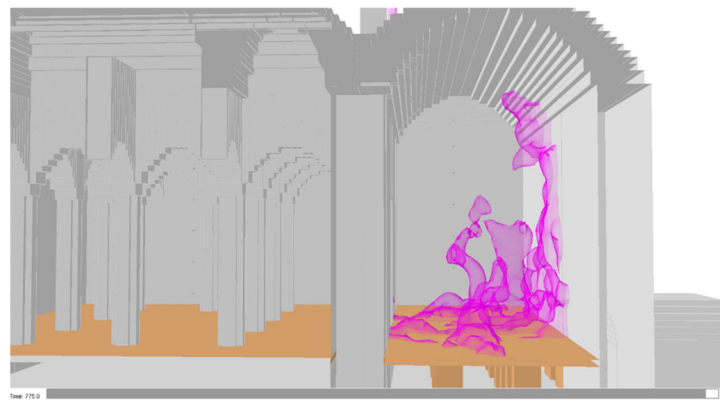
Figure 13. Isosurface with air flow temperatures above 30 °C.
