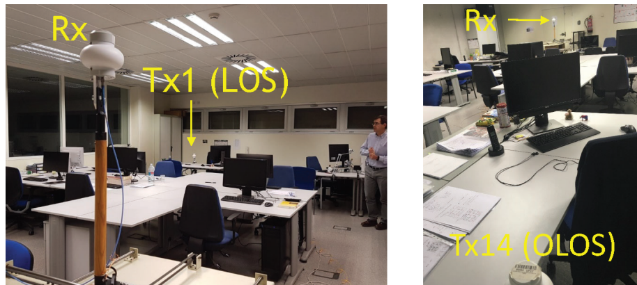
Figure 6. Tx and Rx antennas in positions Tx1 (left) and Tx14 (right) in LOS and OLOS, respectively.
