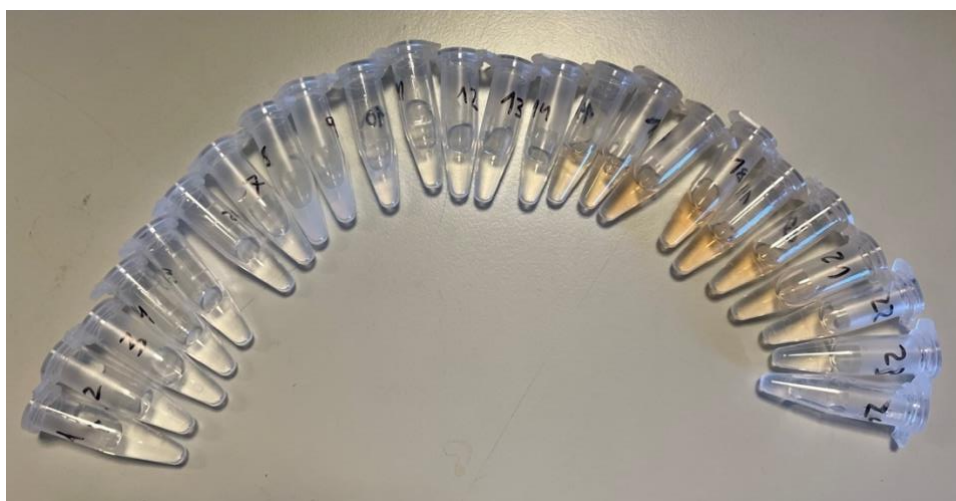
Figure 13. 24 fractions of HRP-loaded LUVs collected after purification with SEC.
