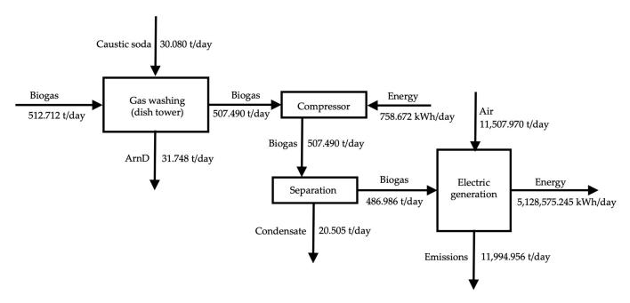
Figure 6. Biogas purification and power generation stage.
