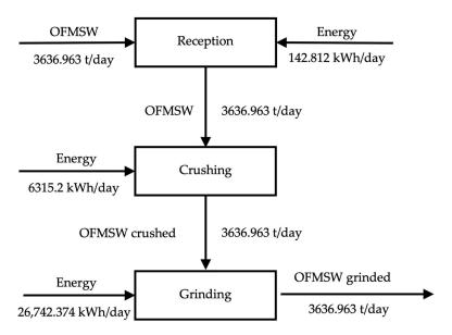
Figure 4. Substrate preparation stage.
