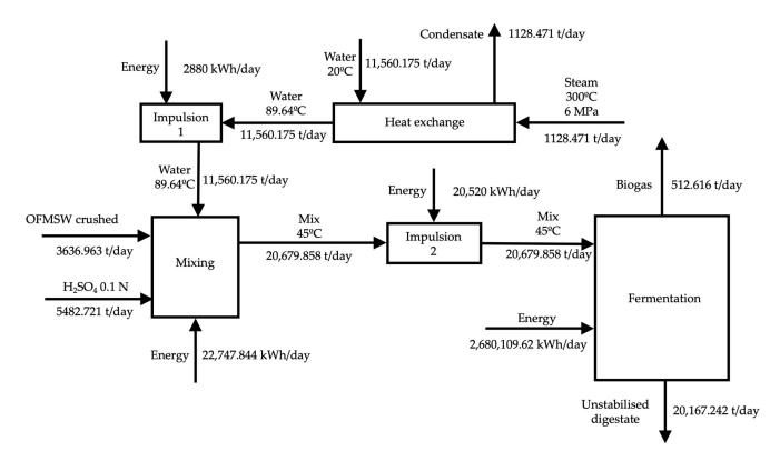
Figure 5. Mixing and fermentation stage.
