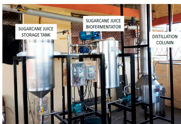
Figure 2. Fermentation of cane juice for bioethanol production in the pilot plant.
